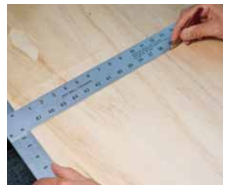
Fig. 1 GRID ON TABLE. A drywall T-square with a four-foot arm works well for laying out a grid on the table. A 12" grid is sufficient for most track plans.
