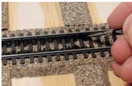
Fig. 4 PAINTING. Paint the ties and insides of the rails the color of the crossing material to
