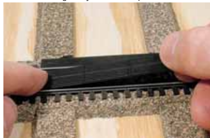
Fig. 5 CUTTING. The Walthers grade crossing can be cut to almost any length needed, so even wide highways aren't a problem.
