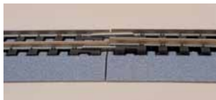
Fig. 4 HIGH-RIDING RAIL. Note how one of these rails is sitting over the rail joiner. Make sure both rails are seated properly.
