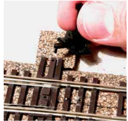
Fig. 3 MOUNTING. Caboose ground throws have a pin that mounts in a hole on the turnout's switch rod. If a matching hole is needed, it's an easy task to drill one.
