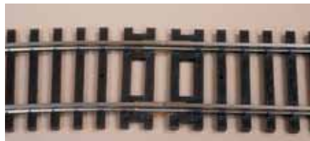
Fig. 2 PROPER JOINT. Track sections should fit together easily, without any obvious gaps in the joint between rail sections.
