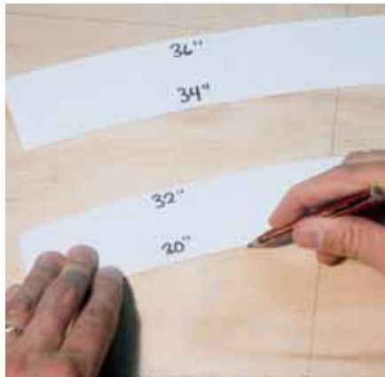
Fig. 2 CURVE CENTERS. Measure to find the center point of each curve, then mark it on the track plan.
