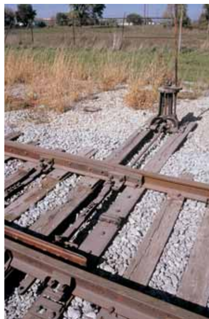
Fig. 1 PROTOTYPE SWITCH STAND. On the real thing, the switch rod connects the points to the switch stand, which is operated by hand.
