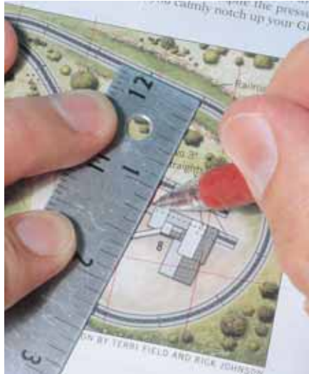
Fig. 2 CURVE CENTERS. Measure to find the center point of each curve, then mark it on the track plan.
