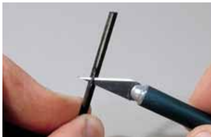
Fig. 6 CARVING. Carve away any material that interferes with the crossing fitting next to the rail.
