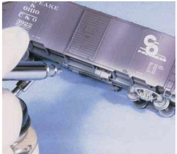
▲ Fig. 5 ROAD DUST. John sprays Earth on the underframe, trucks, and lower portion of the bodies of his cars to simulate dust and dirt kicked up from the roadbed. He changes colors on cars that operate in different regions of North America as shown in table 2.
