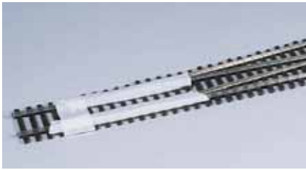
Fig. 3 TURNOUTS. You can airbrush turnouts as you do flextrack, but mask the points and throw bar and paint these areas by hand.
