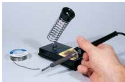
Fig. 3 SOLDERING IRON. A 30-watt pencil-type iron with stand and rosin-core solder will handle most soldering jobs.
