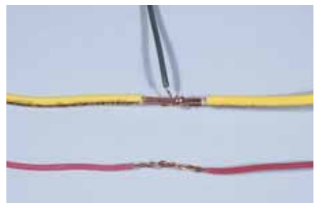
Fig. 4 COMMON JOINTS. For a T-shaped joint, wrap the feeder wire around the main wire. For splices, wrap the wires around each other.
