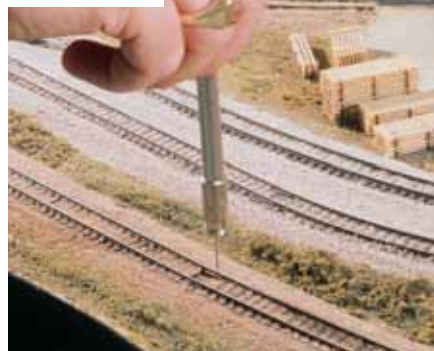
5 DRILLING A FEEDER WIRE HOLE
