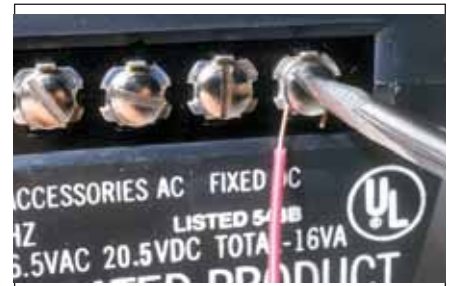
Fig. 2 POWER PACK CONNECTIONS. MRC's Tech II has fixed DC terminals for accessories. Power packs also include variable DC (track power) and fixed AC (accessory) terminals. When making connections, always wrap wire clockwise around the terminal screws.
