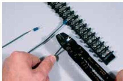
Fig. 8 CRIMPING. Add spade or other terminals to wire by threading them onto the stripped end and crimping them in place.
