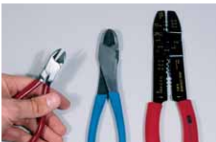
Fig. 2 TOOLS. Small and large (6" and 8") wire cutters and a combination wire stripper/crimper are vital for working with wire.
