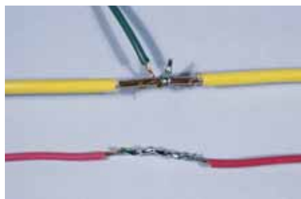
Fig. 6 COMPLETED JOINTS. Joints should be shiny with the solder melted within both wires. The T-shaped joint is a poor joint – the solder only flowed onto the feeder wire, a sign that the larger wire did not get hot enough.
