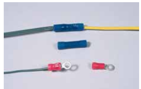
Fig. 9 OTHER CRIMPED CONNECTIONS. Butt joints, as well as ring terminals, can be added using a crimping tool.
